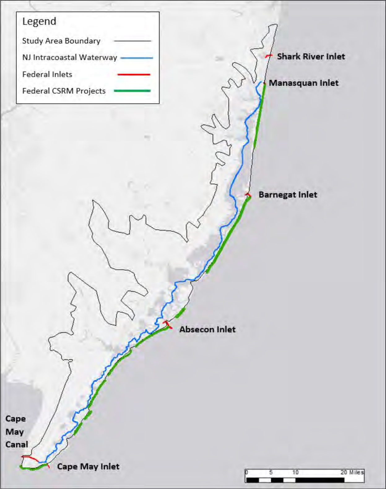
Figure 5-1: Constructed NJ Intracoastal Waterway, Inlet Navigation and Oceanfront CSRM Projects in the NJBB Study Area
